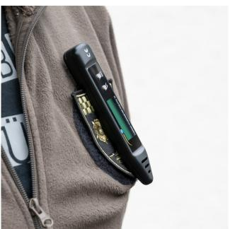
Climate meter with a measuring range of -10 ... 50 °C / Units can be selected / MIN, MAX / Long battery life / LC display / Small and compact design
